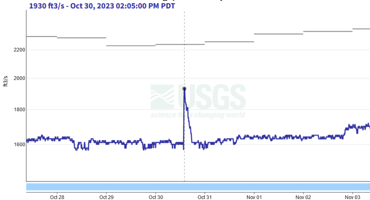
Fig 1. The increase in flow seen below Big Cliff project seen on 30 October 2023.
